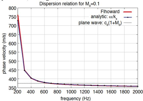
Fig. 1: Numerical dispersion relation compared to the analytical expression in the case of the propagation of an acoustic wave along the wave guide. An ambient Poiseuille flow of maximum mach number  $M_0=0.1$  is present. The graphic shows good agreement of the analytical result compared to Flhoward simulations.
